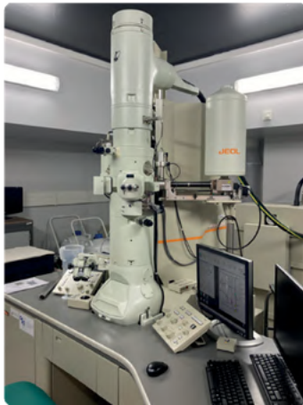
Figure 19: Cryo-TEM setup (left) and example image (right) of the produced LNP using a Herringbone micromixer.
